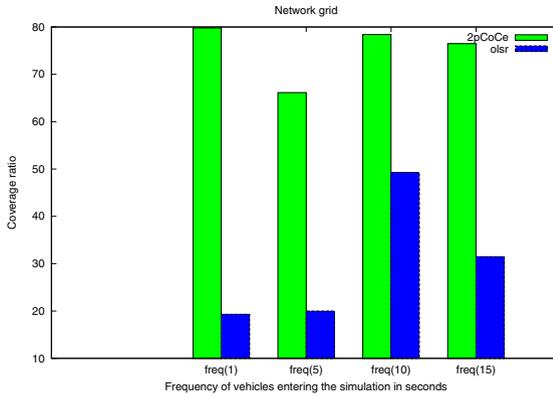
Fig. 2. OLSR Vs 2pCoCe with vehicle velocity at 14m/s
