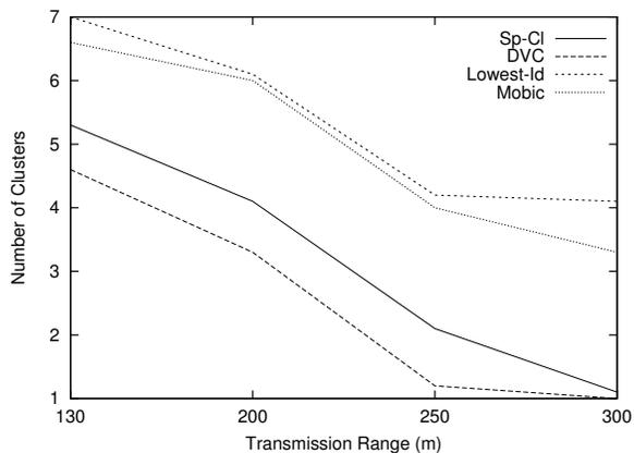
Fig. 5. Average number of clusters for different transmission ranges.
