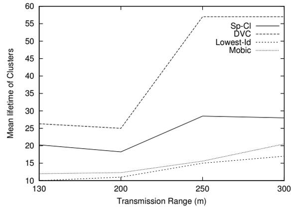
Fig. 4. Average cluster lifetime vs transmission range
