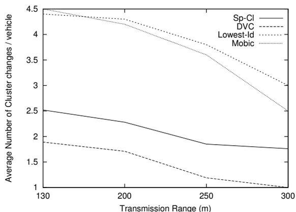
Fig. 6. Clusterhead changes vs transmission range
