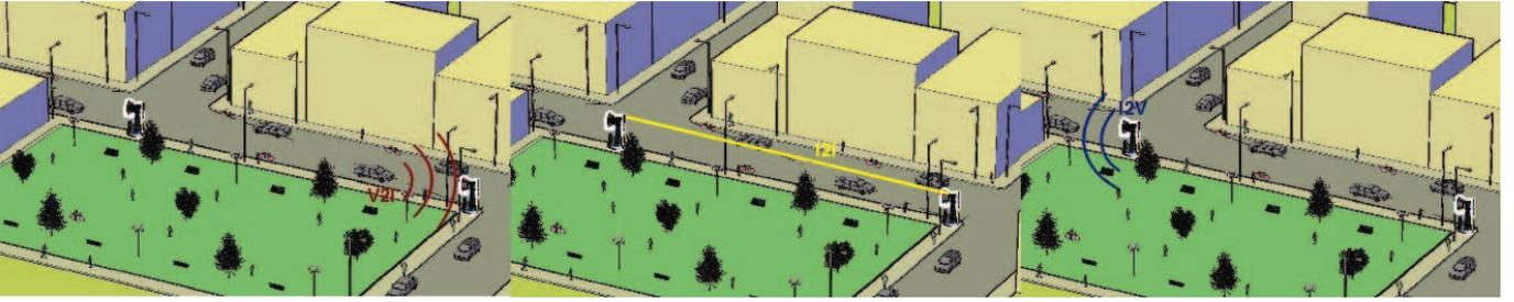
Fig. 2: Application example of *ErouVe* System: A. Vehicle approaching intersection sends a beacon message to RSU (V2I) B. I2I communication for information exchange C. Vehicle receives routing instructions (I2V).
