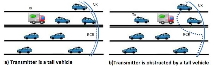
Fig. 3. Reliable communication range is significantly larger for tall vehicles
