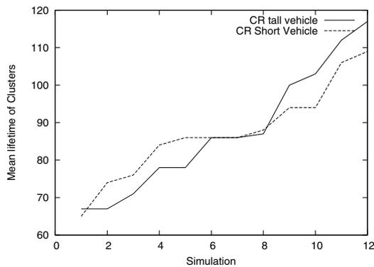
Fig. 11. Height of clusterhead does not affect Spring Clustering's performance, when static communication range is used
